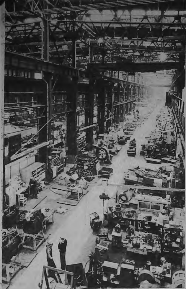
MAIN REPAIR SHOP --Lighted by skylights, the B & M shop contains heavy metal working tools--lathes, presses, welders--all necessary to maintain locomotives and budliners. (Mark Wilson photo)
