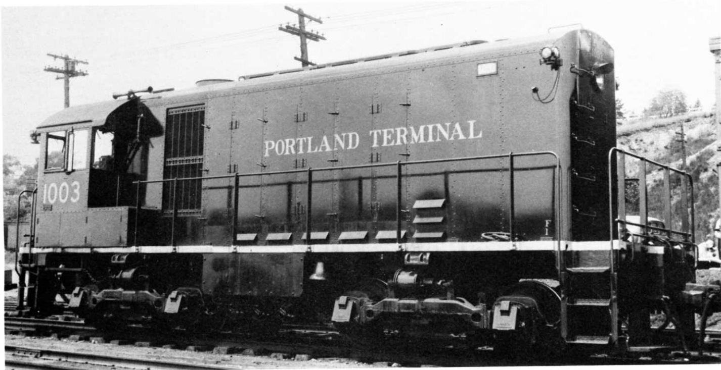
No. 1003 Built 8/28/36 Serial No. 68732 Type S-1 Scrapped 1969
