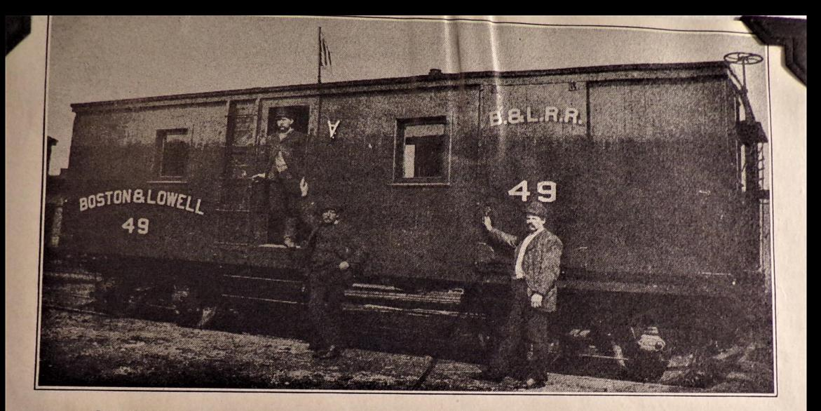
CABOOSE CAR ON THE BOSTON AND LOWELL IN DAYS OF "MILK ROW" A rare picture of much interest to railroaders. Note the flag used as marker on top — also bracket on side of car near center to hold lanterns or marker at night. Coupling pin at end of car is suspended from top to permit man on top to uncouple car. Note also outside brake rigging
