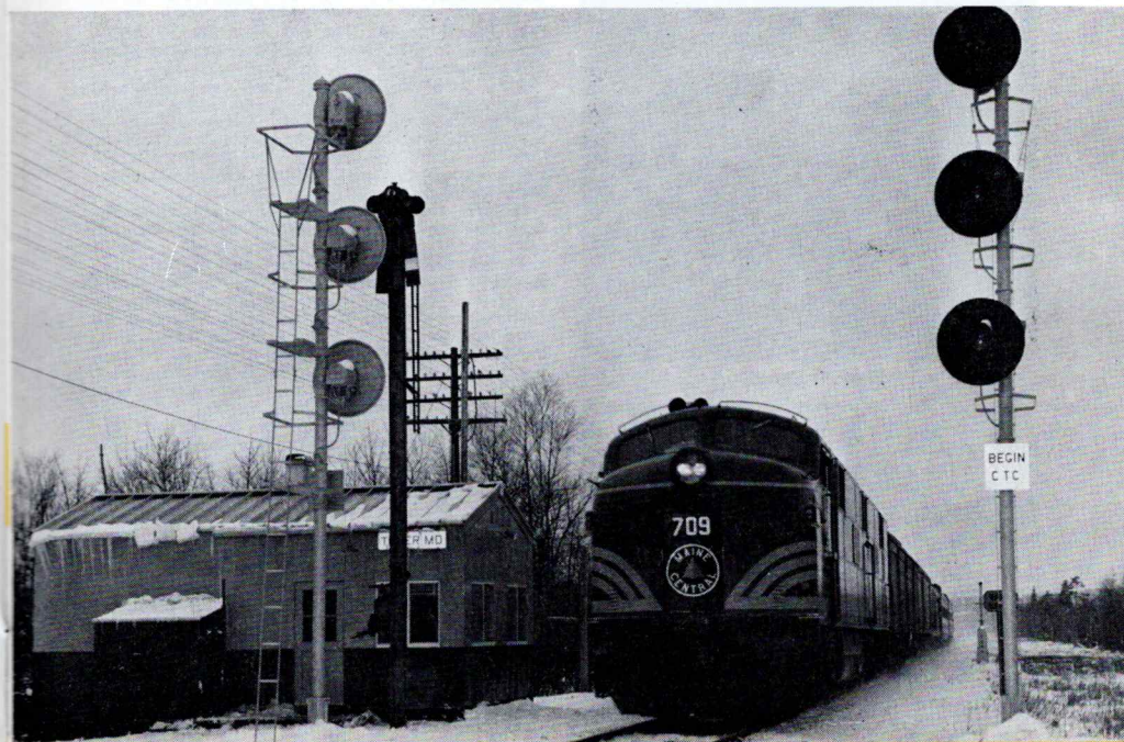
Passenger Train No. 1 completes the first train run between Pittsfield and Hermon after installation of Centralized Traffic Control. An operator in Tower MD, at left of train, controls train operations along the 28 mile stretch of track.
