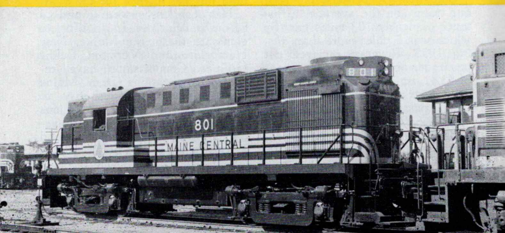
One of two 1,800 H.P. diesel road switching locomotives acquired by our Railroad last year.
