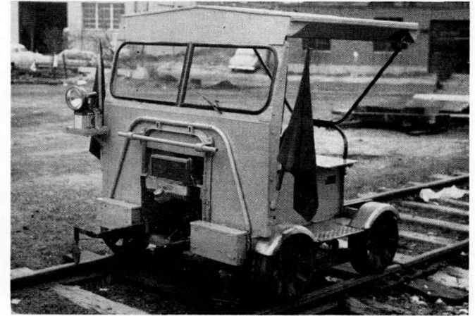
Canopy top and other new equipment for Maine Central motor cars may be easily seen on this Signal Dept. car.
