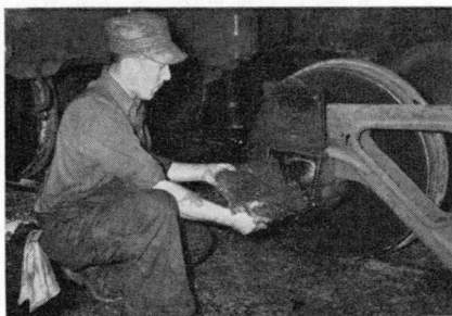
KEEPING THEM ROLLING —Manley Dixon inserts a new-type lubricating pad in a box in the car shop at Waterville.
