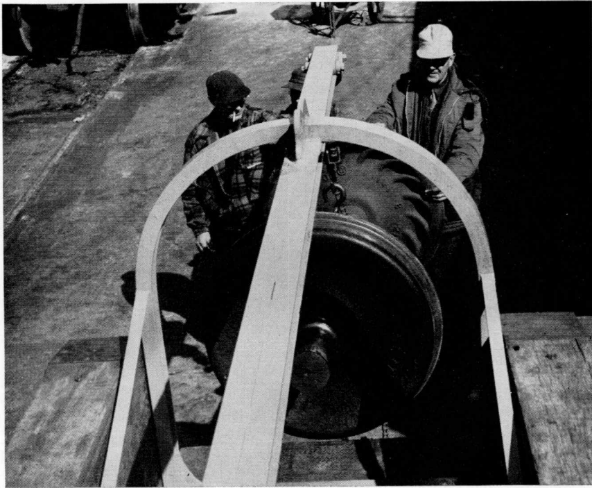
HANDY HOIST SPEEDS WHEEL CHANGES —Freight repairmen at the Waterville Shops demonstrate the ease with which they can handle wheels with the help of a new truck-mounted hoist designed by Freight Foreman Newbert Estabrook, in cap at right. The others are F. R. Case, left, assistant foreman, and carman A. W. Crosby.
