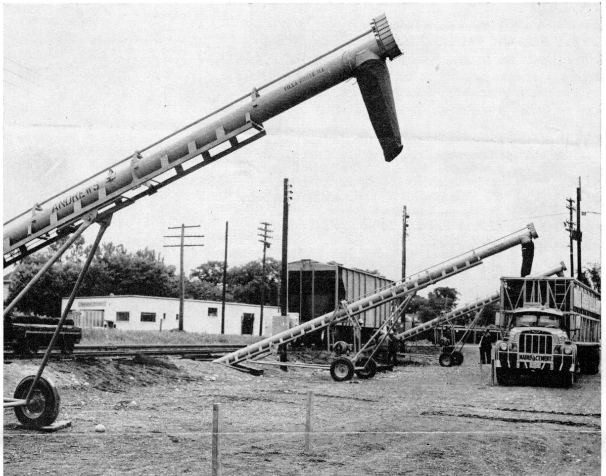
NEW CEMENT FACILITY AT VEAZIE —Maine Central's new cement unloading installation at Veazie is now in full operation. Resembling an artillery battery or a missile site, the new set-up consists of three portable conveyors, one of which is shown in use loading a Maine Cement Products Co. truck from a covered hopper. It is the only machine cement unloading facility of its type furnished by the railroads in Maine.
