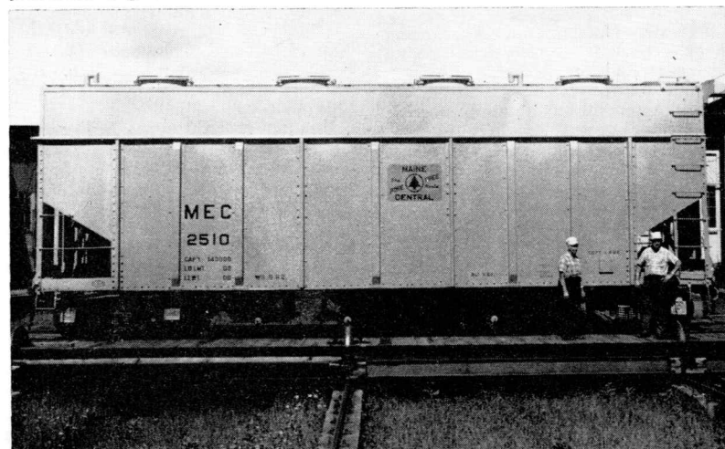
NEWEST CONVERSION —A Norfolk and Western open top hopper, with several modifications, emerges from the Shops in Waterville as a covered grain car to be used between St. Johnsbury, Vt., and the Ralston-Purina plant at Fairfield. The modification includes raising the sides nearly two feet, installing six gates in the bottom and a total of eight loading hatches on top.
