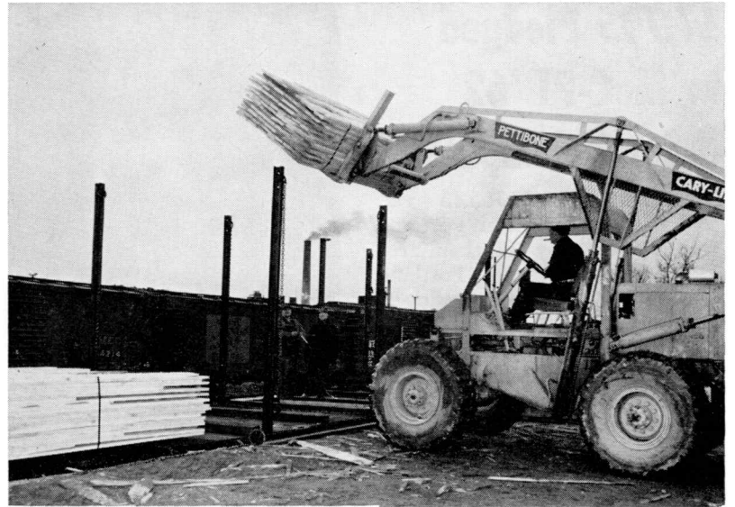
EQUIPMENT IN USE —A car of lumber is loaded at Woodland with a chisel unit provided on a rental basis by the Maine Central.
