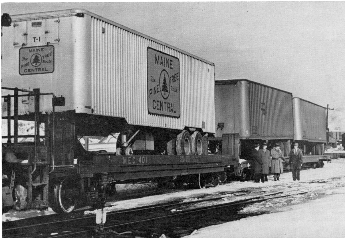
NEW LOW-LEVEL TOFC CARS SHOWN —A full 8½ inches lower than the conventional piggyback car in the foreground are new ACF cars exhibited in Portland in January. Shown as they looked over the equipment are, left to right, George E. Phillips, assistant to the freight traffic manager; R. C. Merrow, freight traffic manager; R. F. Williams, superintendent, PTCO., and M. F. O'Brien, assistant superintendent, PTCO.
