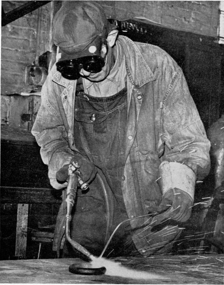
TESTING NEW GLASSES —Welder Albert Wetmore at Rigby shown working on new-type goggle being tried out for "oxy-acetylene" welding and cutting.
