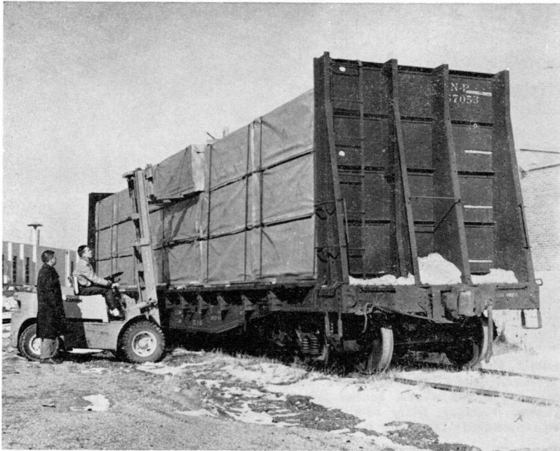
PACKAGED PLYWOOD —Newest wrinkle in the rail transportation of plywood is the "shed-pak" which made its first Maine appearance in January with this car consigned to the Weyerhaeuser Lumber Company, Portland. The load is made up of individually wrapped, weatherproofed bundles. Manager Norman Riviere watches fork lift operator Thomas Flaherty begin the job of unloading the car.
