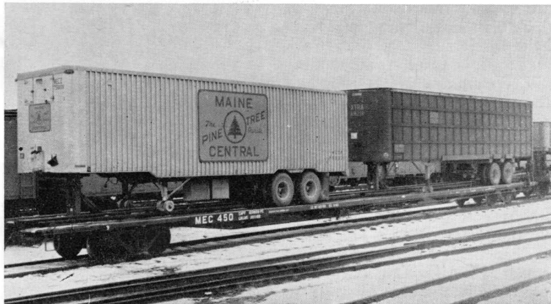
LONGEST ON THE RAILROAD —Purchased this winter and now in service are three of these "long-John" piggyback flatcars, big enough for two trailers, and measuring more than 85 feet end to end.
