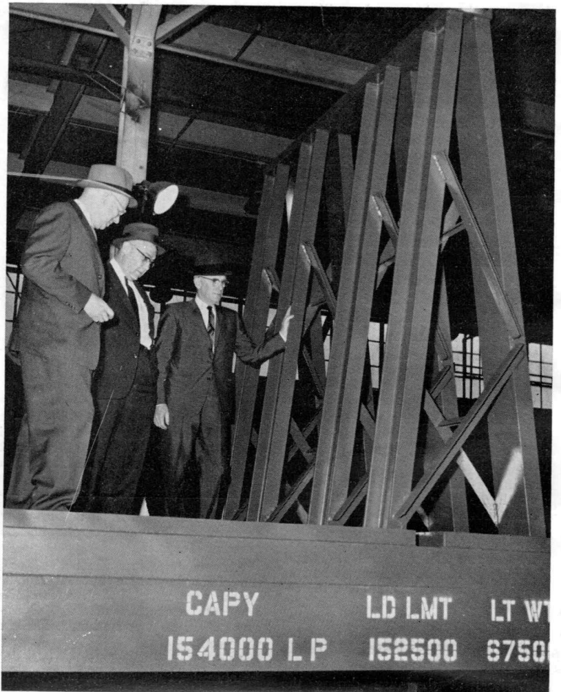
THE "EIFFEL TOWER"—MeC mechanical engineer Richard F. Dole, left, vice president Roy E. Baker, and Vaughn L. Ladd, chief mechanical officer of the BAR., inspect the center bulkhead of the new pulpwood cars. Workmen have named this the "Eiffel Tower" because of its structure and height.
