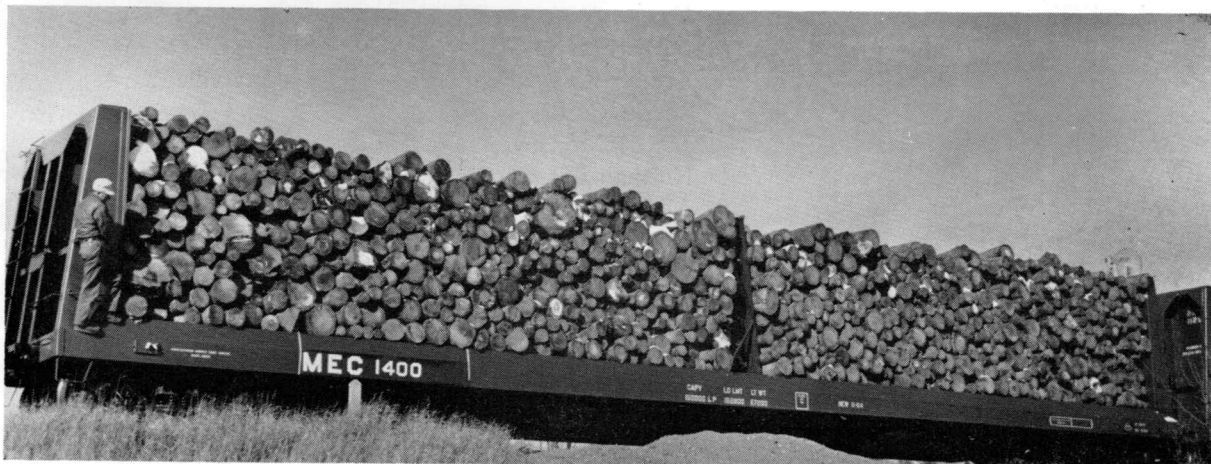
'PAUL BUNYAN' CARS AT WORK—Loaded with 32 cords of softwood pulp, one of the new extra-long, three-bulkhead pulpwood cars is shown at Leeds Junction enroute to the site of the new International Paper Company mill at Jay. Section Foreman E. A. Hall, on the ladder, helps to give us an idea of just how large these new cars are.
