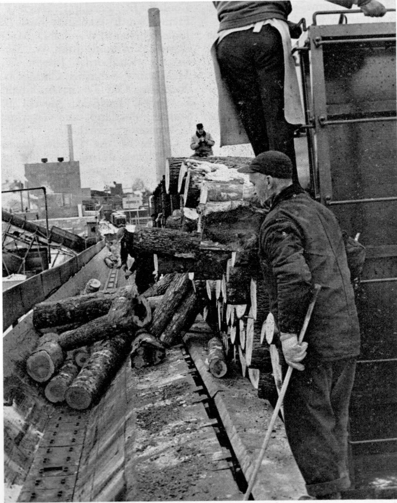
ON THE WAY TO THE PULP MILL —Pulpwood unloaded at the Cumberland Mills of the S. D. Warren company travels down this conveyor to the debarkers and chippers before it is transformed into pulp and finally paper.
