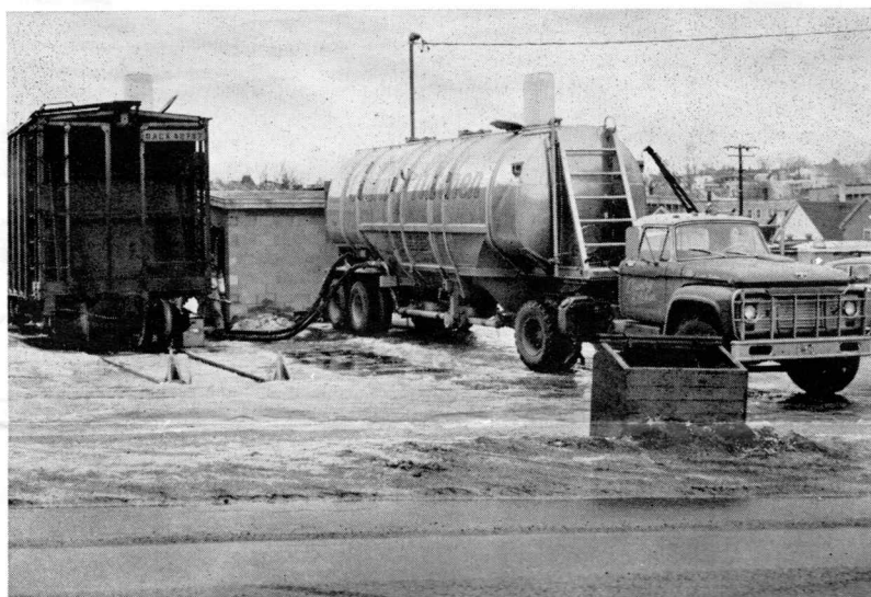
NEW FLOUR-UNLOADING METHOD —Unloading bulk flour by air pressure was begun last month at Lewiston by the Country Kitchen Bakery with the use of specially designed hopper cars and a tank truck. TOP PHOTO shows the machinery in place under the car. The flour passes through hoses to the truck, as shown in LOWER PHOTO .
