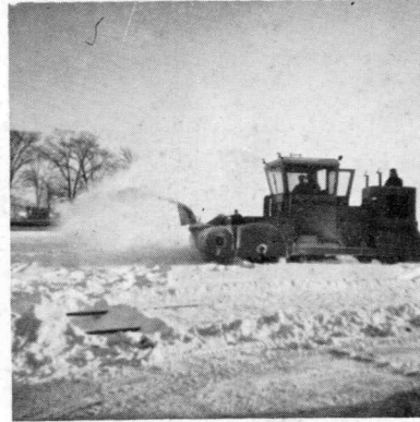
AT WATERVILLE —Pictured is the new Kershaw snow blower working in the Waterville area. This machine is self-propelled and can reverse its direction by the use of its hydraulically operated turntable. It does a fine job of getting rid of the snow between the track down to the ties. Aboard are E. E. "Stub" Murphy, operator, and track foreman Pete Boucher.
