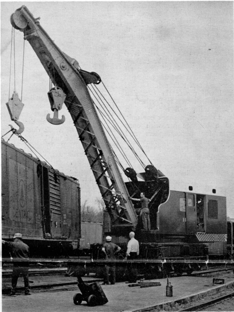
UP SHE GOES —The new crane 160 demonstrates its strength and dexterity by lifting a box car in a try-out at the Waterville Shops.
