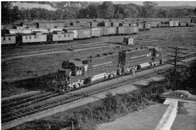
WATERVILLE VISITORS —These two brand-new GP-38's, purchased by the Bangor and Aroostook this Spring, were used on the Maine Central for two weeks in June in connection with studies now being made that will lead to the purchase of several new locomotives by the Maine Central. The big locos pack 2,000 horsepower.
