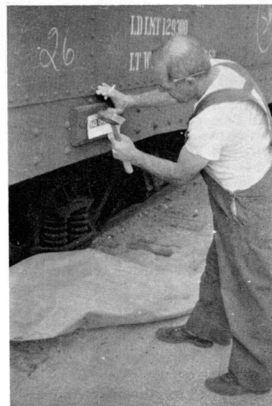
BAD ORDER —Here's Hutch Gravel, Car Inspector, tagging a bad one. This is Hutch's daily task to sort the bad from the good cars for our surrounding industries in the Waterville area. (Photo by Doucette)
