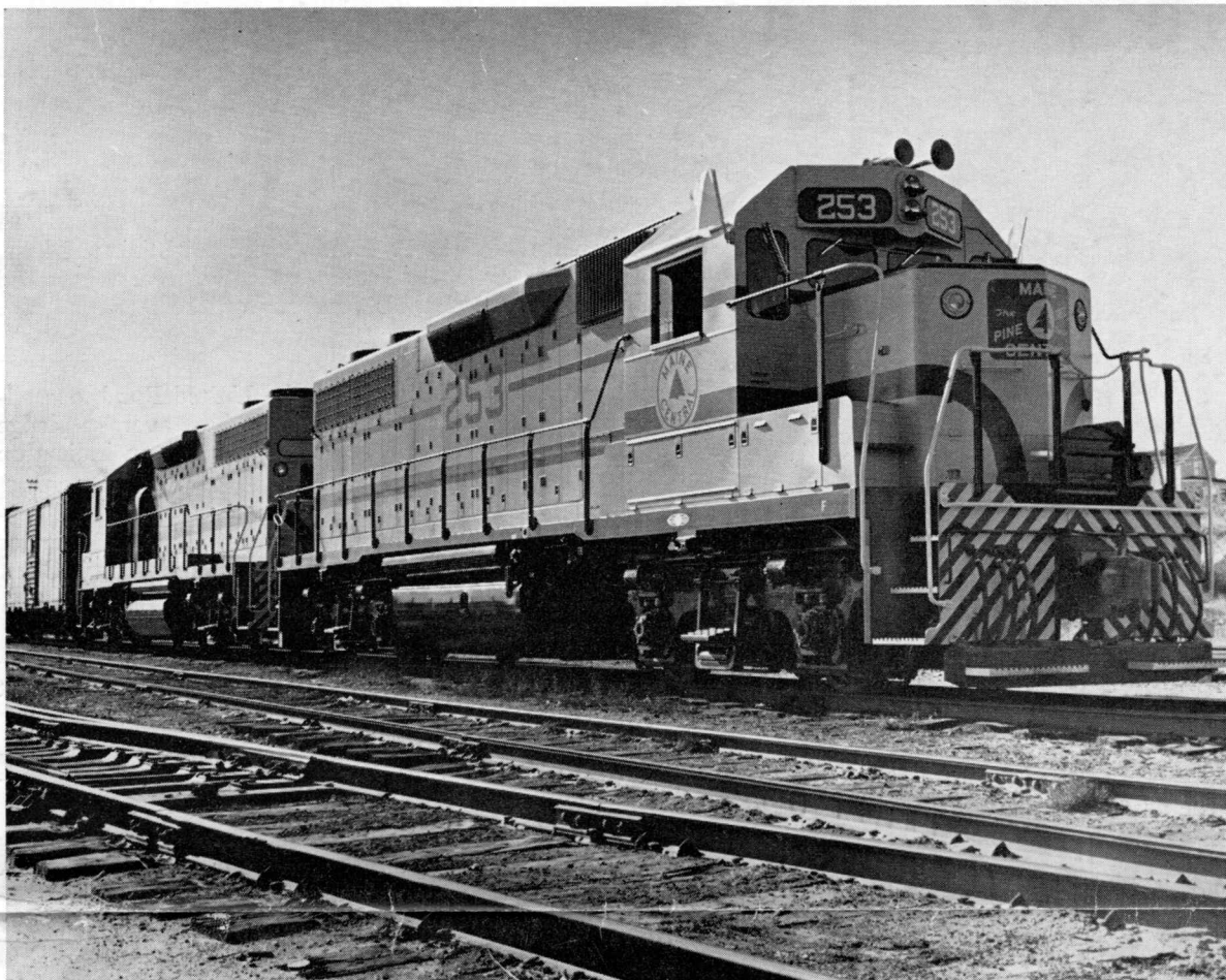
FIRST UNITS ARRIVE —The first of 12 brand-new diesel locomotives, numbers 253 and 254, arrived in St. Johnsbury November 19 and were placed in service immediately. Built at LaGrange, Ill., by the Electromotive Division of General Motors, the big new engines boast 2,000 horsepower and weigh 260,000 pounds. Total cost of the dozen new diesels is more than $2,000,000.
