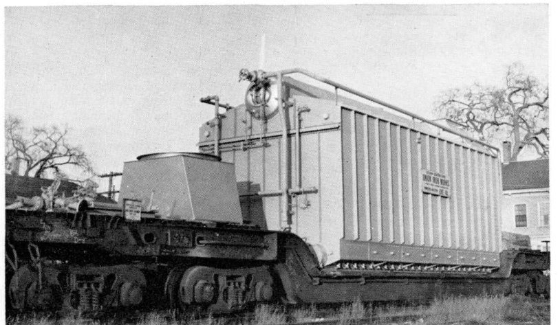
A HEAVYWEIGHT FOR ROCKLAND —This 51-ton steam boiler, consigned to Marine Colloids, Inc., Rockland, rode a depressed flatcar from Erie, Pa., to its Rockland destination last month. Tipping the beam at a total of 282,400 pounds, the heavy car and its huge load constituted one of the heaviest burdens ever hauled into Rockland by the Maine Central. (Rockland Courier-Gazette photo)
