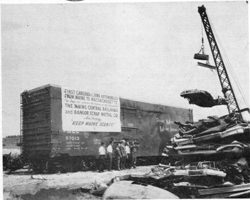
JUNK AUTOMOBILES . . . MAINE'S NEWEST EXPORT —The first carload of junk automobiles is loaded at the Bangor Scrap Metal Company destined for Everett, Mass., where metal is reclaimed for re-use. This car, developed for wood chips, will carry about 40 crushed autos. State officials see a solution to Maine's growing junk car problem in this method.
