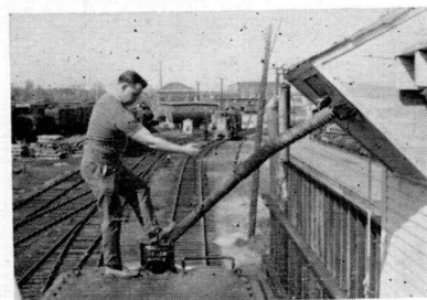
This is the man behind the scene. Ed Sargent is sanding and fueling engines upon arrival at Waterville Engine House.
