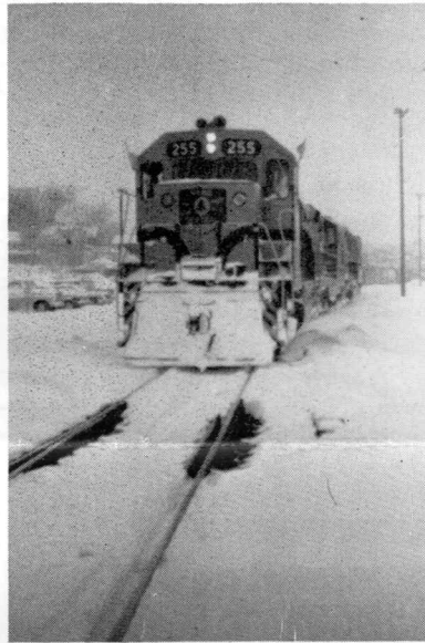
ITS OWN PLOW —This is advance B-12 as it arrived in Waterville prior to setting off and picking up. The engines—one of the new GP-38's—did some plowing of its own on the way to Waterville.
