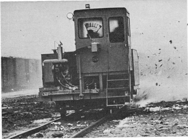
MeC JET IN ACTION —The new "Hurricane" jet snow blower at Rigby—there's another at Bangor—clears a foot of snow from a yard track after one of the January storms. What's left is bare ground, with maybe shreds of snow, but little more.
