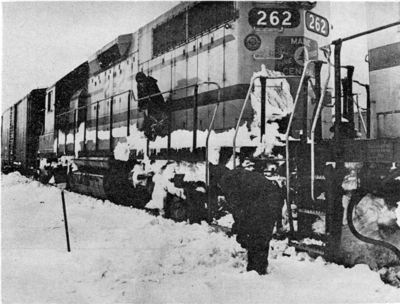
Workers remove snow from locomotive 262 as a train is made up. Snow build-up under the engines proved troublesome during the storm, actually cutting down traction. It was necessary to remove the accumulation several times during a trip.
