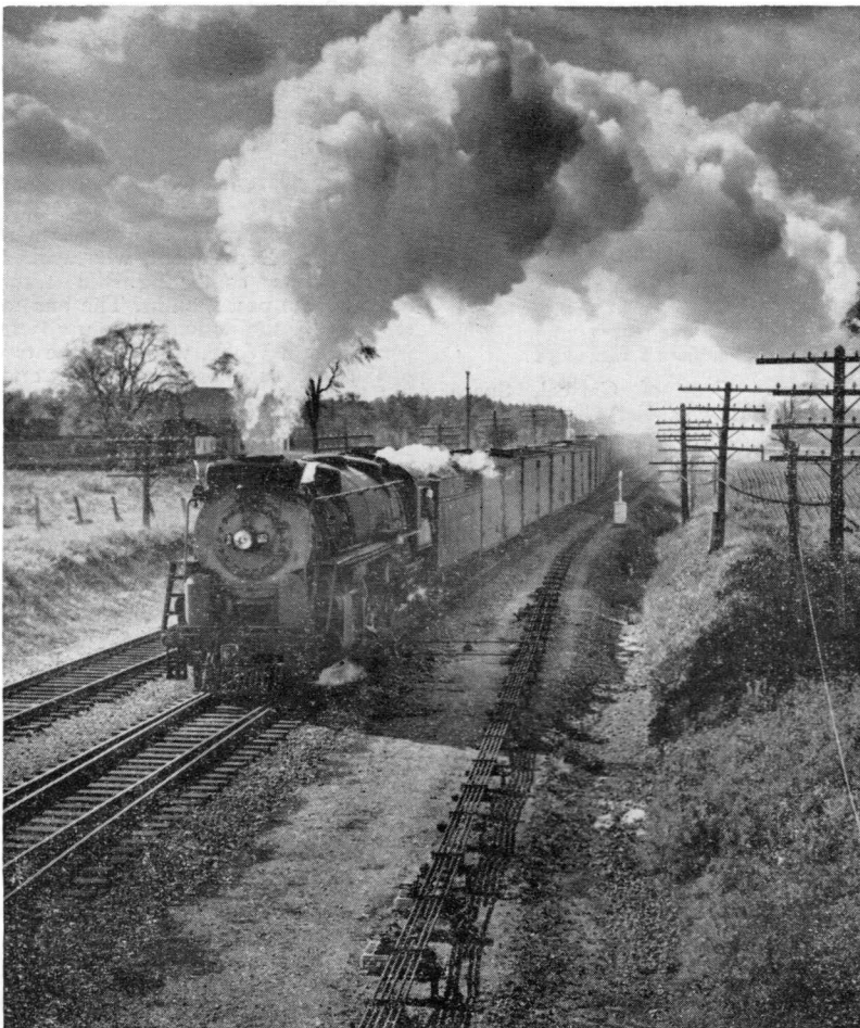
NOTHING PRETTIER —This photo, from the collection of Gardner M. Roberts, Chief Photographer for the Portland Press Herald and Evening Express, was made on the main line of the Bangor-Portland run, at Riverton in Portland. The locomotive was Maine Central No. 652, a powerful 2-10-2 Santa Fe which hauled heavy freights. It was originally one of the Boston and Maine Railroad's 3000-class, purchased by Maine Central in 1937, and scrapped in 1950.
