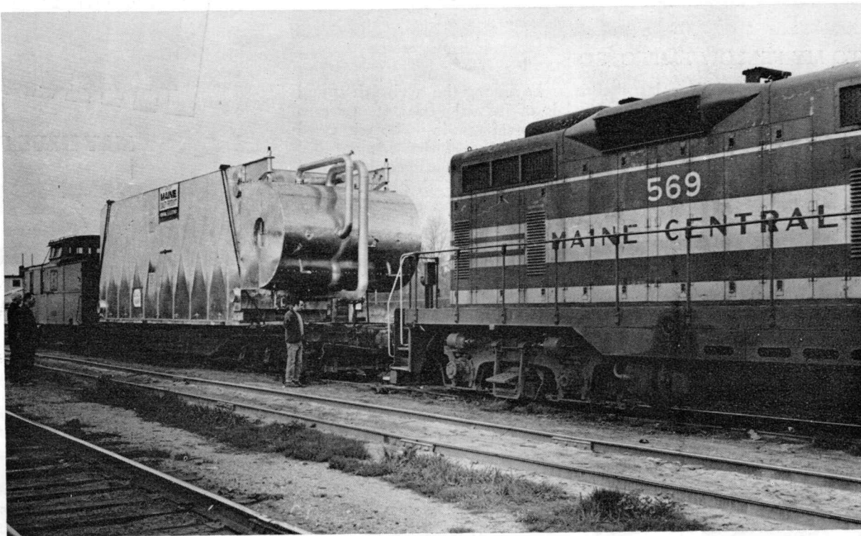
BIG JOB FOR MAINE CENTRAL —Maine Central—with an assist from the Portland Terminal Company—moved the largest generator ever built by the General Electric plant, South Portland, last month. The big, close-clearance unit required a special car and supervision during its trip from Maine to a southern city.
