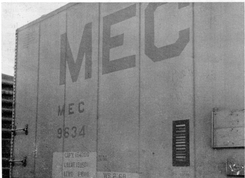
LIVING COLOR —would show this ACI label to be vivid shades of red and blue. The labels, made of retroreflective material have been applied to both sides of MEC Car 9634 as these markers will with all cars in the fleet before the deadline January 1, 1970.
