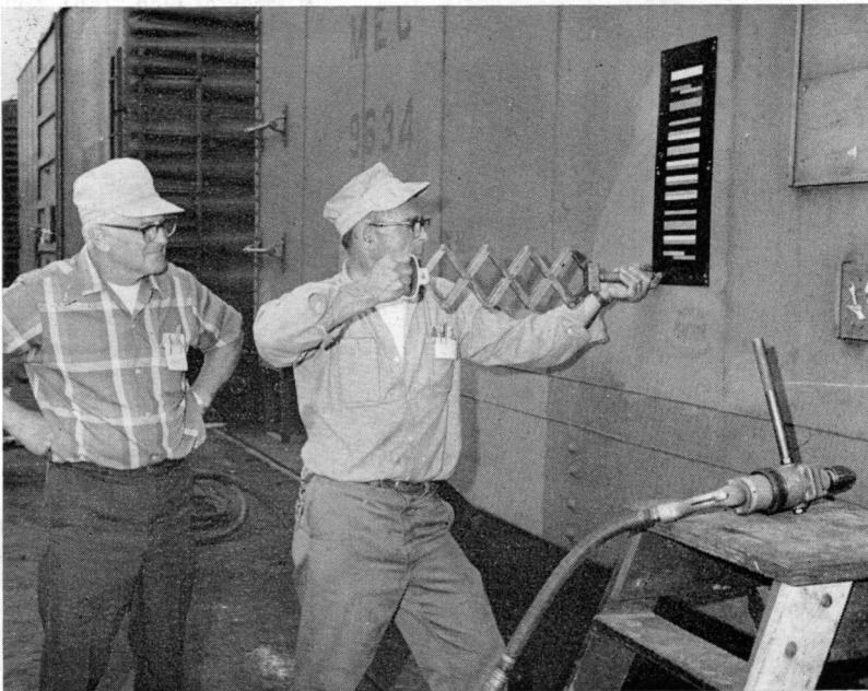
APPLICATION—Holes are drilled in the sides of the car and plates applied by use of a hand-pop riveter with a 1/4" snap-off rivet.
