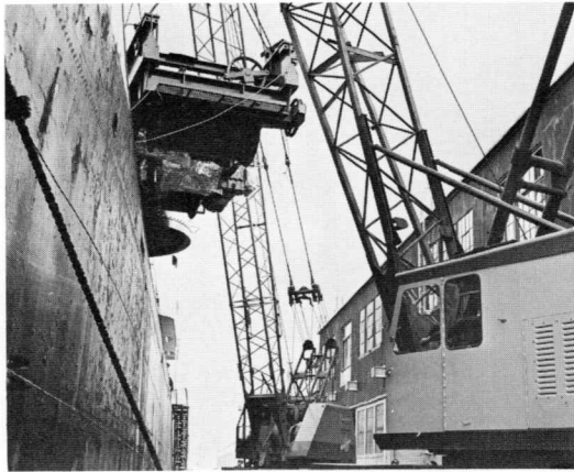
One of the largest sections of the giant crane is eased down to the flat-car between the grips of a 50-ton and 60-ton crane.
