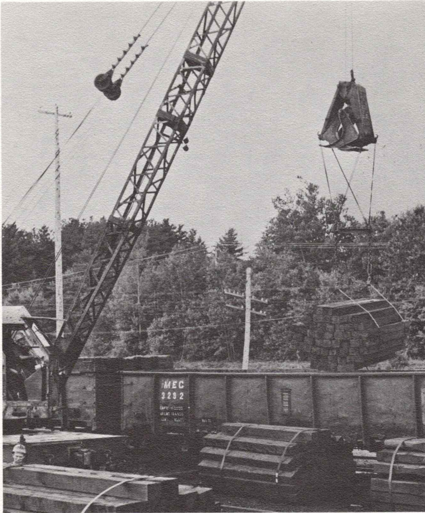
Seasoned and treated hardwood cross ties are loaded into a Maine Central gondola.
