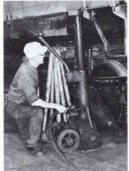
Waterville Shops employee Ralph Roberts preparing a boxcar for installation of trucks which have been modified with new roller-bearings wheel assemblies.
