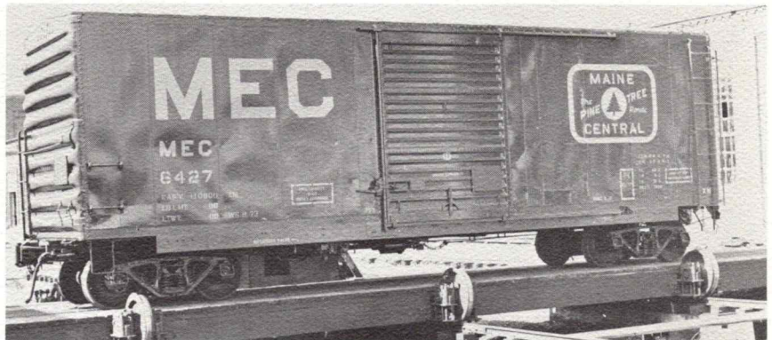
MeC 6427 is one of the current 50 forty-foot box cars being rebuilt at Waterville Shops. These cars are completely upgraded for paper service, with new all steel interior lining with lading strap anchors, hardwood flooring, 8-foot wide doors and high capacity draft gears. In addition, new roof, under-frame reinforcement, roller bearings and the latest design brake equipment result in a car that is virtually brand new.
