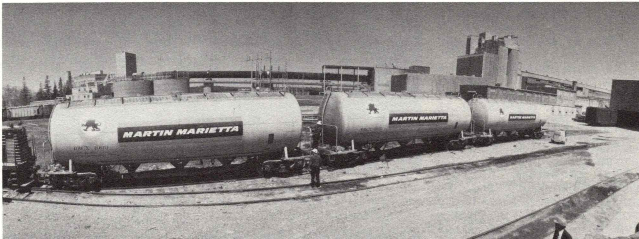
Martin Marietta's air-activated 530-barrel tank cars used to transport cement from Thomaston to the Company's terminal near Boston, Mass. This photograph, taken with a wide-angle lens, shows the plant with its 520-foot rotary kiln in the background.
