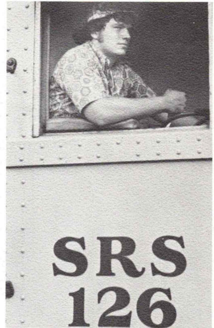
The Sperry Rail Service car is powered much the same as a locomotive with diesel-electric power. The car is used to test rail for internal flaws. Story on page 4.
