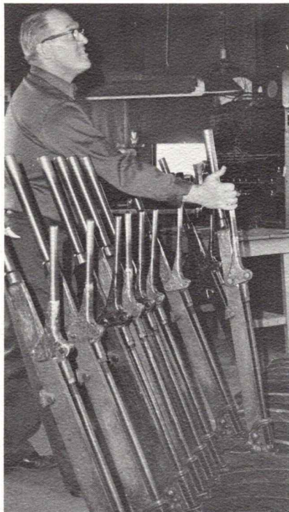
Joseph Weingaertner, Portland Terminal Company tower operator, throws switches in Tower 2 before the tower consolidation took place. These hand-thrown switches are the last of their kind on the Maine Central system.
