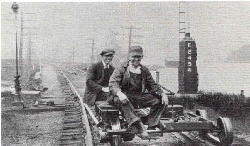
This photo was taken at Lambert Lake many years ago. The man on the front has been identified as a Mr. Hunter and the man on the rear is signalman Jack Ryan. This motor car has a two cylinder engine on each side of the front wheel which is attached to the crank shaft. You have to push it to get it started because it is in gear all the time. Photo from L. E. Brown.
