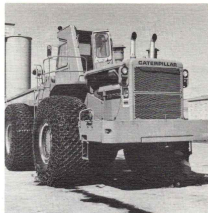
Arnold Machinery and crew put these heavy duty link chains onto the 39 x 38 rubber tires of the new excavating machinery. They have prepared it for delivery to the Martin Marietta Cement Corp. at Thomaston. This equipment was shipped in by rail on two flat cars from the Caterpillar Tractor Company. When finally assembled enough to move over the highway, it was so tall that several places had to be detoured around to avoid low hanging overhead wires.
