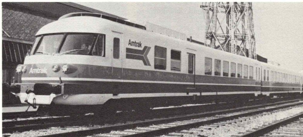
This French built, 125-mile-per-hour turbine powered train marks Amtrak's first tentative step into the high-speed passenger service of the future, operating between large population centers.
