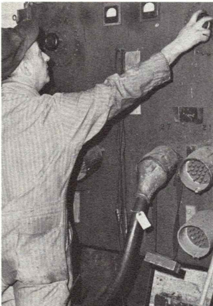
Shapleigh Allen, electrician, tests multiple-unit jumper cables on test stand.
