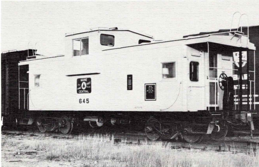
In November 1973, Maine Central placed in service the first of a series of new "wide vision" caboose cars. The side walls of the monitor are as wide as clearance will permit in order to provide maximum visibility. Maine Central will purchase one new caboose of this design each year.
