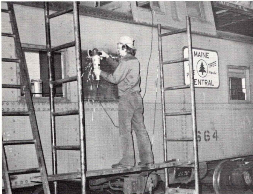
Robert Michaud, carman helper, works on the caboose rebuild program at Waterville Shops. This steel caboose, built in the late 1930's was purchased from the Western Maryland Railroad in 1962. The rebuild includes: relining with insulation, repair of undercarriage, installation of a toilet, grit blast and a new paint job. The program calls for 4 caboose rebuilds a year.
