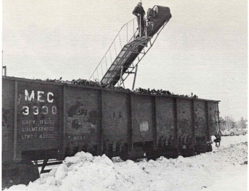
Shredded steel produced from junk cars by National Metal Converters at Leeds is loaded into Maine Central Railroad cars to be shipped to steel mills.
