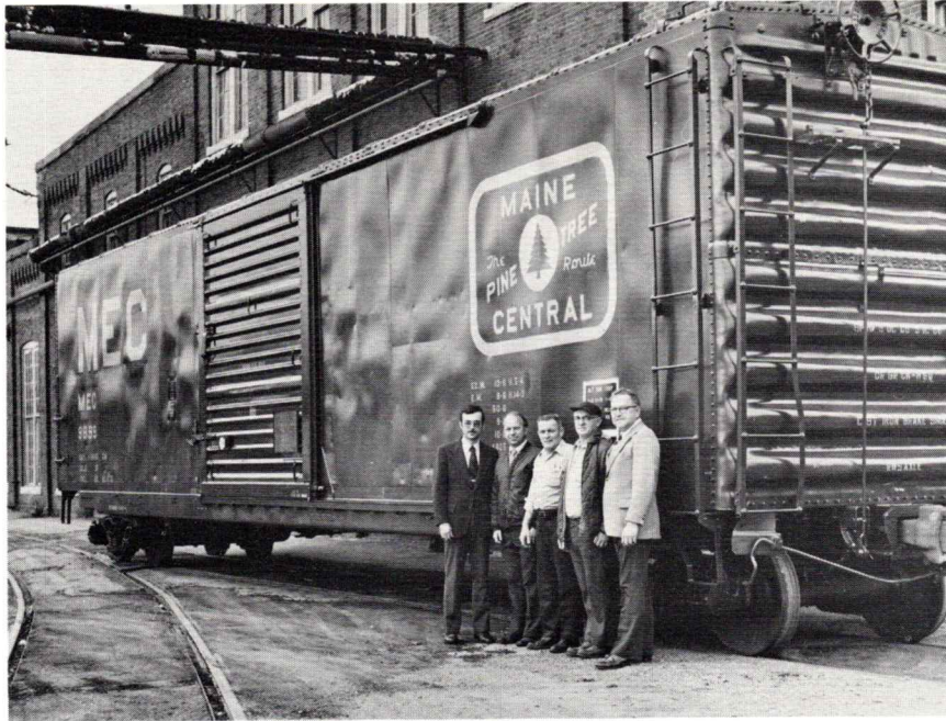
The last car in the stretch program at Waterville Shops was completed in November 1975. One hundred old 40-foot cars have been completely rebuilt and stretched to 50 feet. Left to right are: David Crovetti, mechanical engineer; Donald Dickey, general shop foreman; Glen McCarrison, foreman; Basil Thompson, foreman; and Wade Richardson, shop superintendent.
