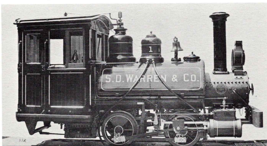
S. D. Warren's No. 1 narrow gauge engine as it came off the Baldwin assembly line in 1895. Photo from H. L. Broadbelt collection.
