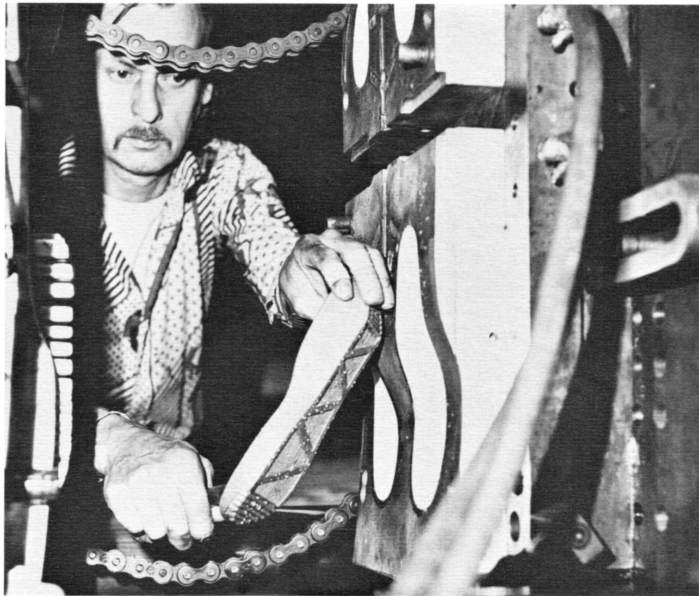
A J.V. Components worker removes a unit sole from the mold at the plant in Conway, New Hampshire.
