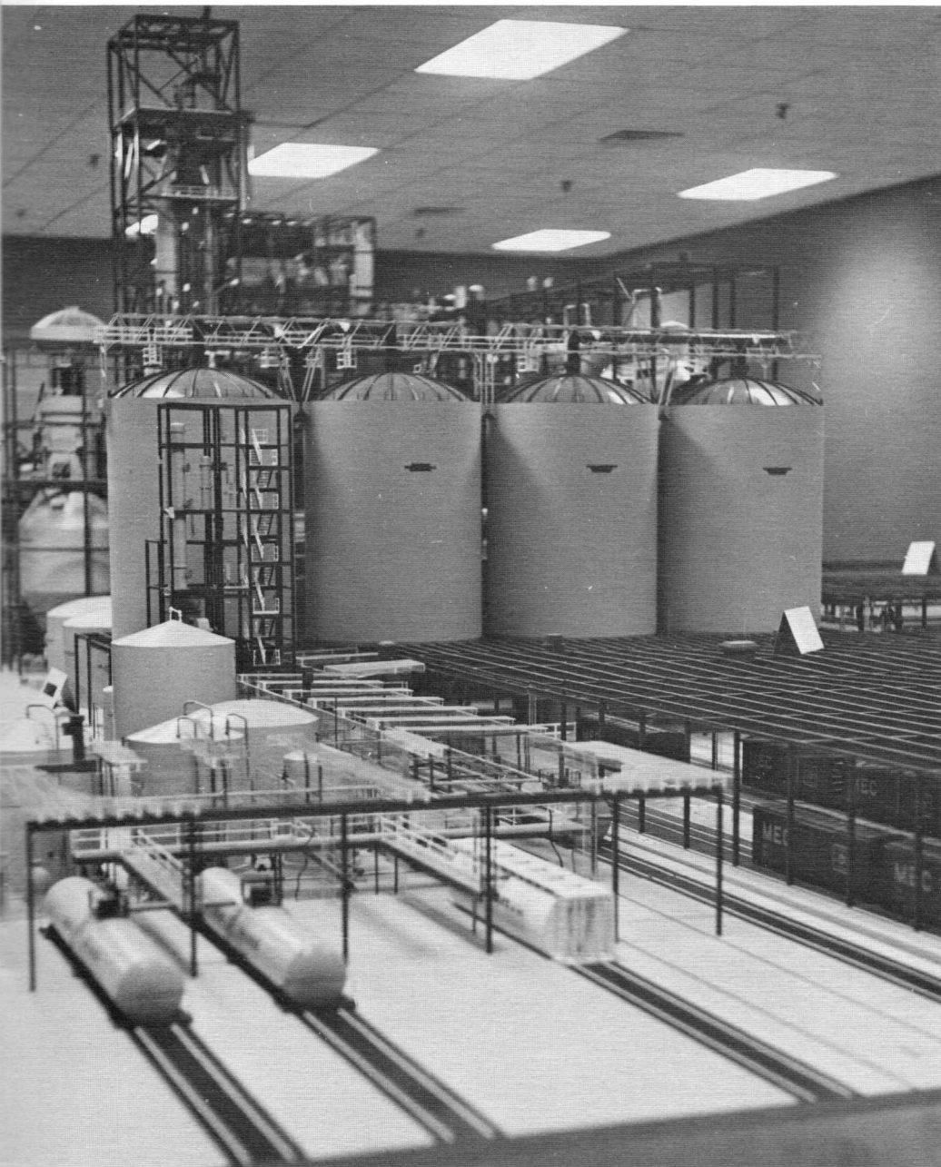
A model of Scott Paper's new pulp mill complete in every detail. The model, which fills an entire room, was very valuable during plant construction and continues to be used during operations.
