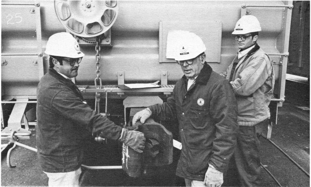
Left to right, inspectors Peter Reny, Roland Boulette and Dave Denton check the coupler and cushioning device on Maine Central's new boxcars. Photo by Bruce Harmon, FMC Corporation.
