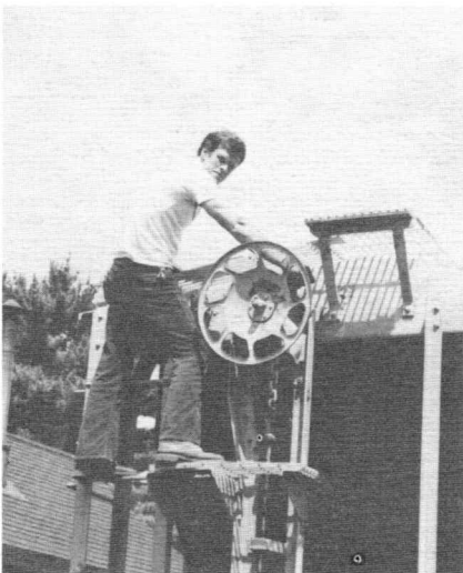
Ron now releases the hand brake. His body is clear of the brake wheel and chain and he maintains a secure footing and handhold. Also remember that the safe method for climbing for a hand brake is to climb the side ladder and then cross over to the end ladder and brake platform.
