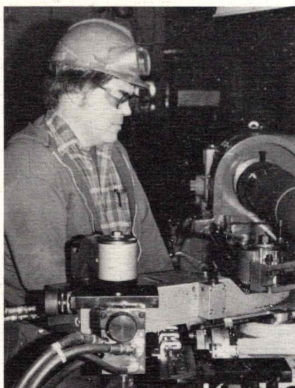
Safety glasses with side shields are worn by Bill Trafton while working at Waterville Shops. Note the goggles ready to be used for other jobs that require their use.
