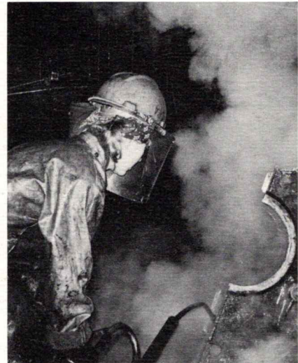
A full face shield is a must when working the Vat Room at Waterville Shops. Laborer Wanda Runnells protects her face from burns with this shield.
