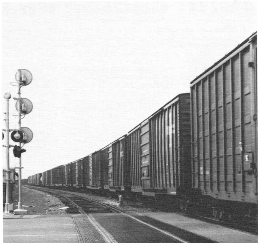
Twice as costly, but requiring less maintenance and with a longer life than bituminous crossing surfaces, rubberized crossings are being evaluated in Portland, Waterville, Brewer and Brunswick.
