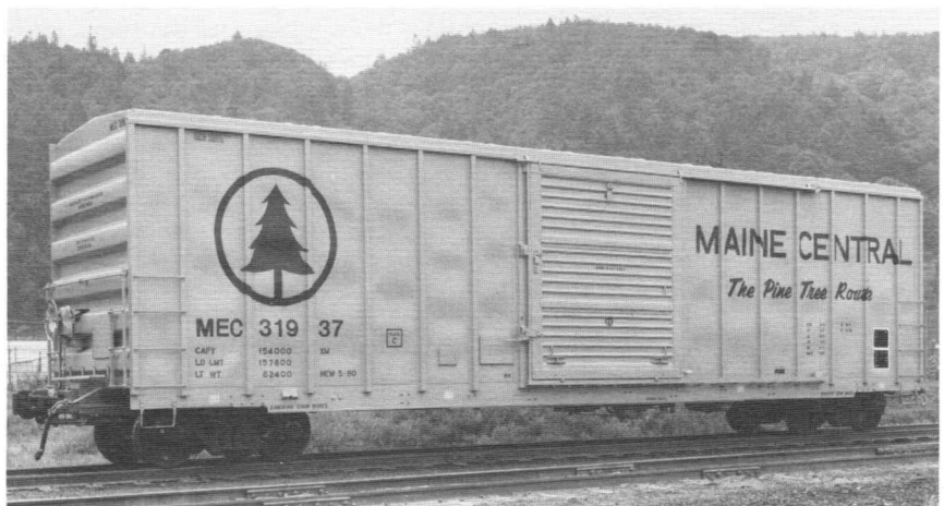
One of the 450 new box cars acquired by Maine Central is 31937, one of a series built by FMC in Portland, Oregon. The 75-tonners were repainted by the manufacturer for Maine Central after the original buyer cancelled their order.
