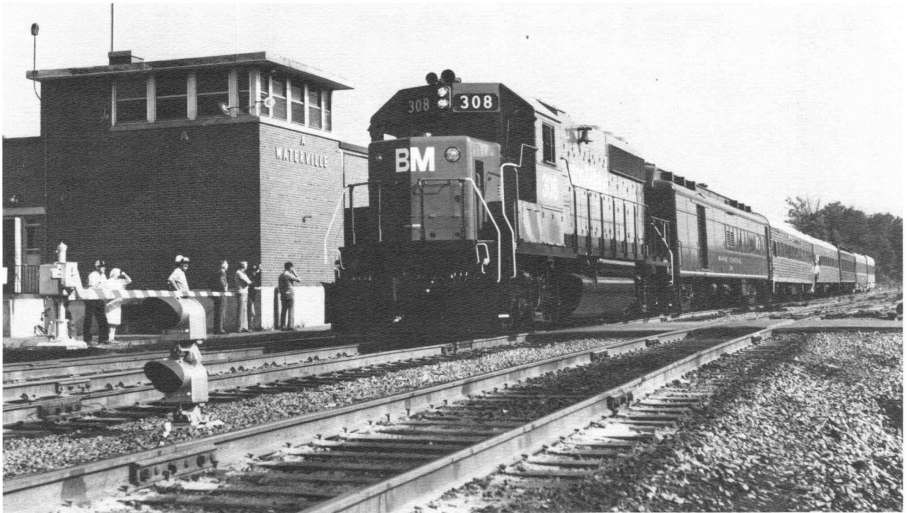
The inspection special slips past Tower A at Waterville, at the heart of the Maine Central system. The consist was a B & M GP40-2, 3,000 HP locomotive, a Maine Central auxiliary car, two former Amtrak coaches refurbished by MEC, the 1924 Pullman Maine Central business car, a D & H lounge car and the D & H business car. (Ron Johnson photo)
